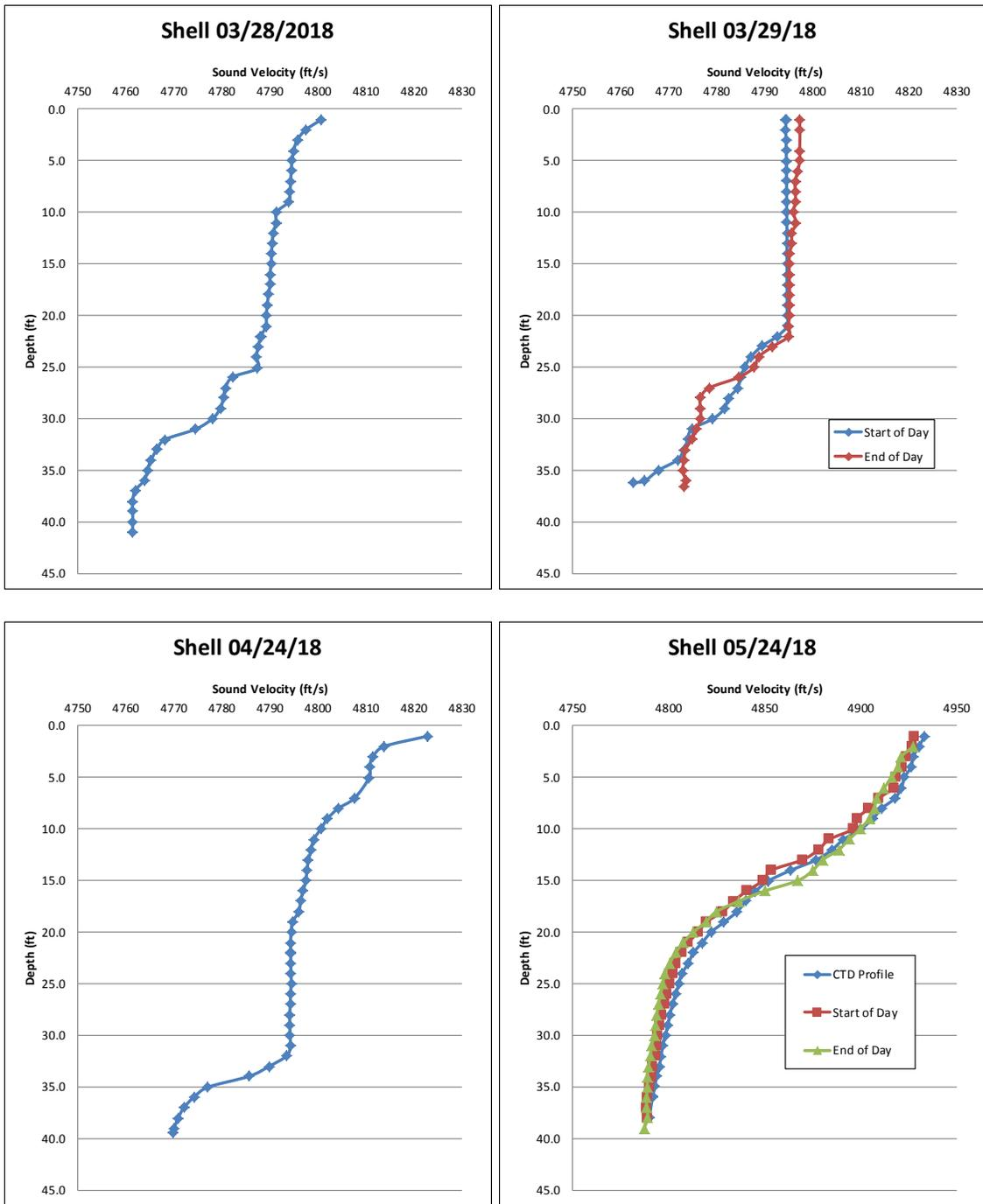
**Figure F- 1: Shell Lake Sound Velocity Profiles (Calculated and Measured).**
