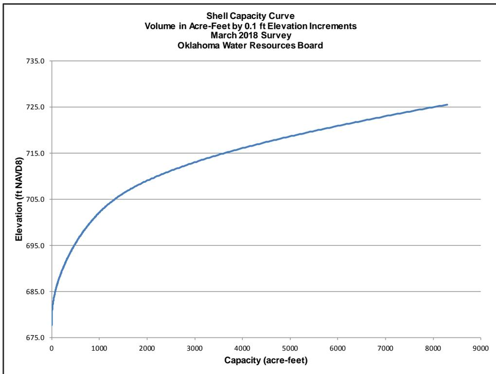
**Figure A- 6: Cumulative Capacity Curve for Shell Lake.**
