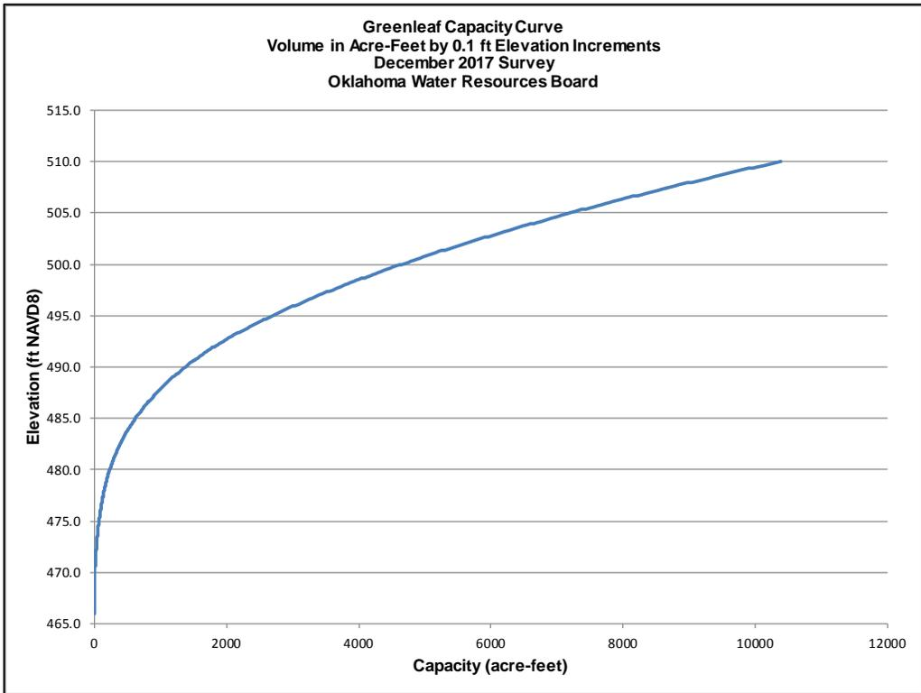
**Figure A- 4: Cumulative Capacity Curve for Greenleaf Lake.**
